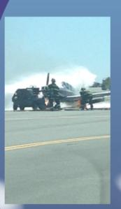
Small Aircraft flew into Logan Airport and the brakes locked up. After 30 minutes ignition temperature was achieved and caused the plane to ignite.
