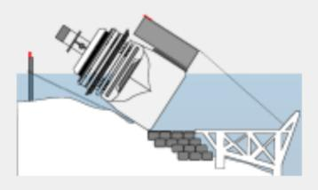
2. Underwater support system platform to catch Costa Concordia as it rolls upright.
