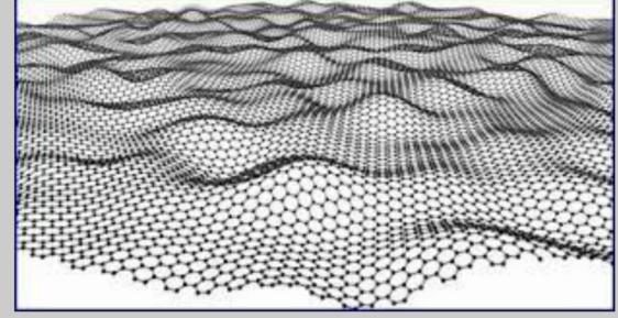
The thinnest, The lightest, and the strongest material discovered. the best conductor of heat at room temperature and also the best conductor of electricity known.
