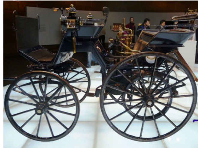
the first 4 wheeled automobile (was actually just a stagecoach made to hold an engine)
